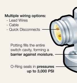
Three magnet design provides **snap action** and solid contact pressure, eliminating 'contact teasing' and 'contact chatter' in high vibration applications.
