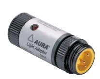
The Aura Light Adapter provides LED position confirmation on any N/O GO Switch using a 3, 4, or 5 pin Mini-Change connector.
