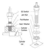
Models 73-76 - 5/8" Diameter Torque Jam Nuts to: 15 lbs-ft to achieve seal at 2,000 PSI 25 lbs-ft to achieve seal at 5,000 PSI Do not exceed 30 lbs-ft
