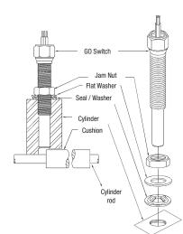
Model 77 - 3/4" Diameter Torque Jam Nuts to: 20 lbs-ft to achieve seal at 2,000 PSI 65 lbs-ft to achieve seal at 5,000 PSI Do not exceed 75 lbs-ft
