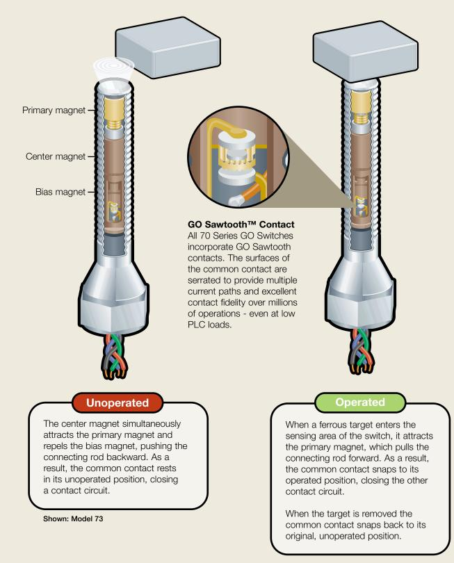
Permanent magnets never lose their strength, even when threaded into ferrous metal.
