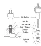
Models 71 & 72 - 3/8" Diameter Torque Jam Nuts to: 15 lbs-in to achieve seal at 2,000 PSI 30 lbs-in to achieve seal at 5,000 PSI Do not exceed 45 lbs-in
