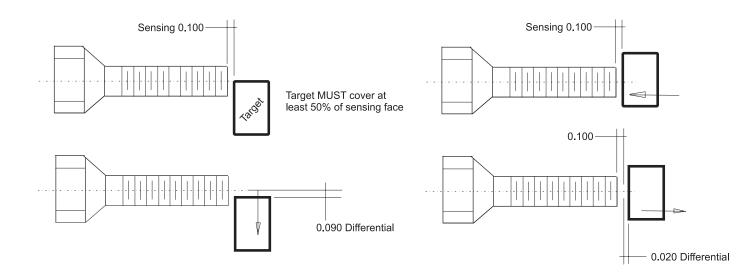
The measurements shown are nominal and can vary as much as .030-.050" depending on the material and size of target used in the application. As you can see, the best scenario for least differential is to orient the switch and target as shown in **Orientation B**. However, in this application, the possibility of getting debris between the switch and target must also be considered.
